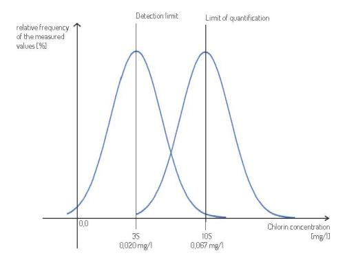
Drawn in blue are the possible measurement results of the meter with their relative frequency at different chlorine concentrations. This is called a measured value distribution. It is gaussian, i.e. the middle measured value is most likely to be measured and the probability of measuring corresponding values decreases towards higher and lower measured values up to 0% probability.
