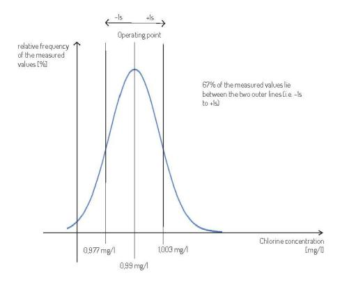
Here a problem becomes apparent: If a measuring device achieves this precision in only 2 out of 3 cases, the statement for a practical application is rather low. Therefore, the confidence range was still given at 1.00 mg/l free chlorine (+- 0.021 mg/l): In 95 out of 100 measurements, the measured values ranged from 0.979 mg/l to 1.021 mg/l. The operating point for this is 1.00 mg/l free chlorine, as this is a typical working value for swimming pool applications.
